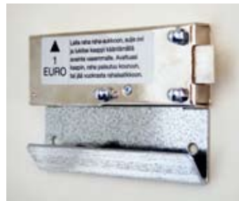
Abloy Exec 1€ deposit lock (not for doors under 197 mm high) or collecting coin lock (not for doors under 400 mm high). Coin lock doors equipped with pullback spring.
